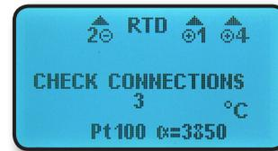
Only a calibrator with PIE's patented 2, 3 & 4 wire detection makes troubleshooting sensor wiring quick, easy and automatic. This is much simpler and faster than going through the process of testing each pair of wires to figure out which, if any, connection is loose or which wire is broken.
