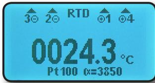
Here is an example where connections are made to a 4 wire sensor and the 311Plus indicates that only Wires 1, 2 & 4 are connected. There may be a loose connection or a break in wire 3 somewhere between the sensor and the 311Plus.
