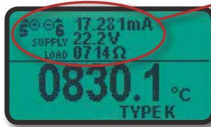
With *LoopScope* running the 830 simultaneously displays the sensor input along with the loop current, power supply voltage and loop load in ohms.
